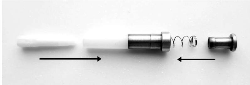
6] Place the pocket clip over the click mechanism and insert into the heel end of the pen and using your preferred method (press/vice/lathe etc) press firmly into place
