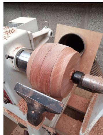
When we have got it roughly round we mount a jacobs chuck on the tailstock and drill another 45mm hole approx 10mm deep so we can turn the box around when we have finished the sides and bottom:
