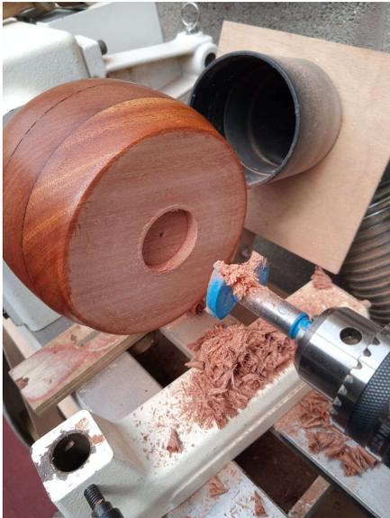
When we have done this we then use a 3.5mm drill bit to drill just into the bottom of the drawer section.
