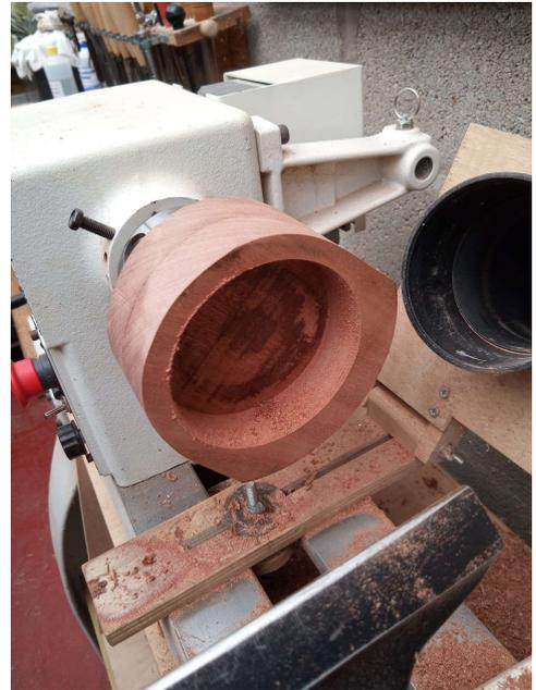
Take extra care with the drawer - as it is not round it will be out of balance on the lathe – start at a slow speed and gradually increase to get a stable suitable turning speed.
