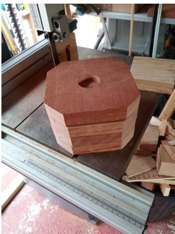
The screw is installed and we have trimmed off the corners on the bandsaw to save a bit of mess and make turning a little easier.
