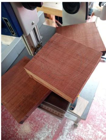
You will see that we have marked out with a compass 2 circles which will be the inner and outer walls of the drawer.
