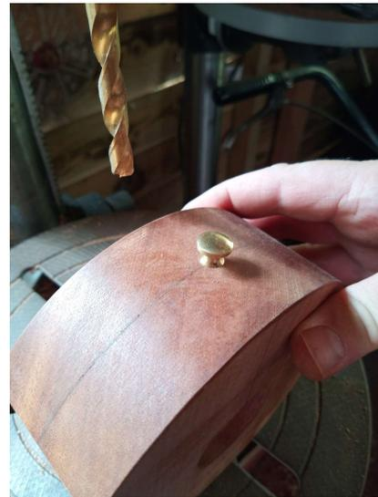
The final part is to take the box back to the pillar drill and drill the 45mm hole all the way through the top of the box, mark and drill the pilot holes for the coffee grinder mill kit and bolt it on.
