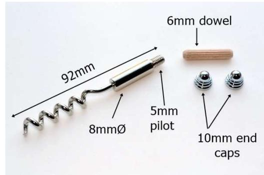
To make the kit 3 drill holes are required, one at each end of the blank 8mm long 6mmØ and one in the centre to a depth half way through your blank 5mmØ
