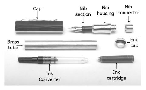
You will require a blank at least 85mm long drilled out to 10mm and trimmed down to 79mm. Once the brass tube has been glued into the drilled blank it can be turned using a bushing set either on a mandrel or between centres as you prefer.
