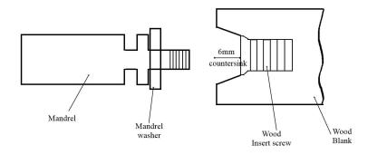
NB: For acrylic parts you will need to tap an M8 thread directly into the blank using a 7mm drill and M8 tapping tools
