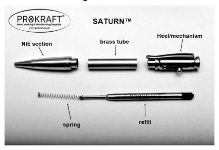
You will require a blank at least 45mm long drilled out to 9.5mm and trimmed level with the brass tube. Once the brass tube has been glued into the drilled blank and trimmed it can be turned using a bushing set either on a mandrel or between centres as you prefer.
