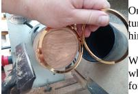
Once marked you can hollow the inside of the lid, making sure you turn the pencil mark away completely to obtain a flush fit between the hinge leaf and the wood inside the box.
