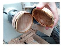
Once the inside is complete you can do a test fit to ensure all the parts fit together correctly as above. Then turn the part round and finish in the same manner as the lid.
