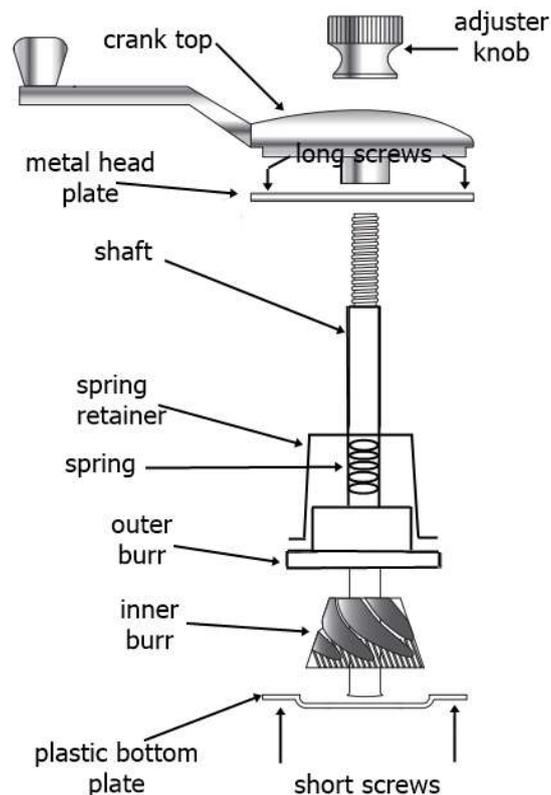
DO NOT fully tighten the adjuster knob and force the handle or you may damage the grinder burrs.
