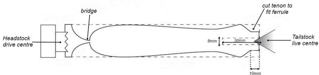
5] Finish by pushing the ferrule over the tenon and gluing the handle shaft of the kit into the handle. The ferrule does not need to be glued in place, the main scoop will prevent it from slipping off and the ferrule will prevent the wood from splitting from internal pressure from the shaft.
